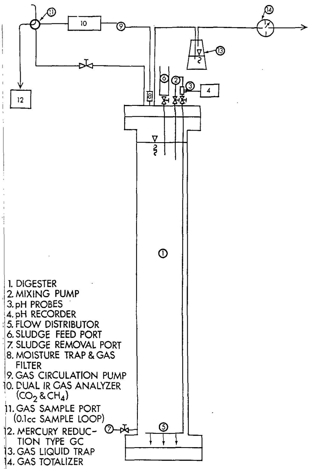
Figure 2 Schematic representation of the 5 liter on-line test digester.
